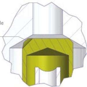
The Integral Snubber Type Syphon eliminates damage due to pressure surges. A slot is providing an auto reset of the deflector tube.
