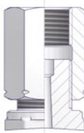
Swivel Nut (Welded Nipple Design)
