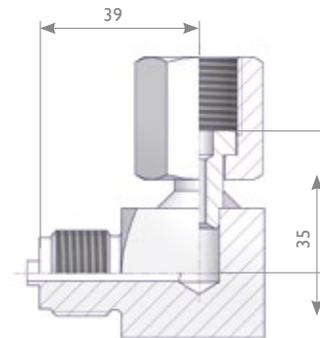
Max. allowable (Working) Pressure (PS): Type 1 10,000 psi / 689 bar
