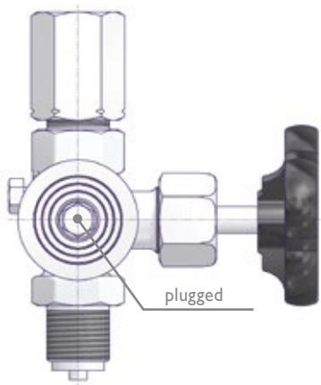
Valve with Test Flange Ø 40 x 5
